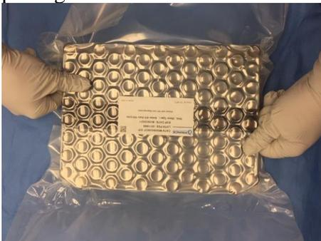
5. If one or both of the interior most bags (bags# 1&2 for triple packaged or bag# 1 for double packaged) show loss of vacuum, the product shall be marked as non-conforming.
