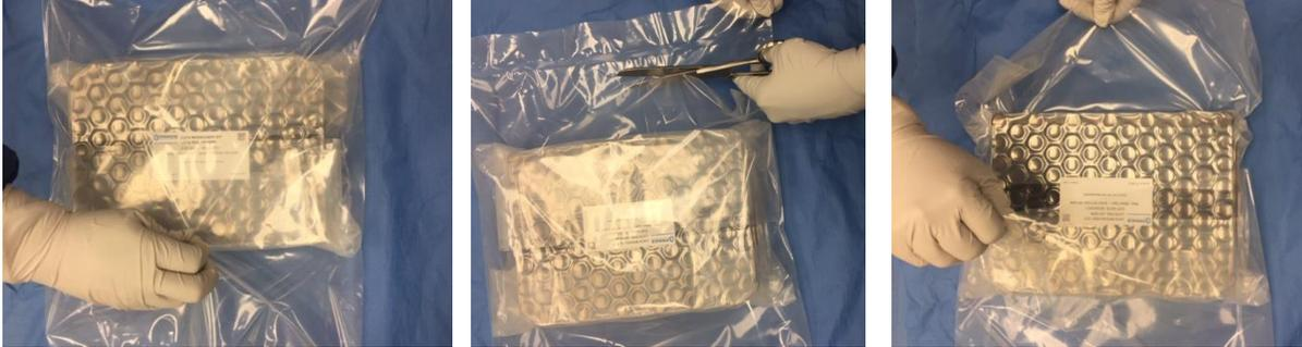
4. Loss of vacuum is only a concern for either or both of the interior most bags (bags #1 & 2) for the triple packaged vials or for the interior most bag (bag #1) for the double packaged vials.
